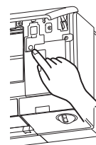
Emergency operation switch (E.O. SW)
